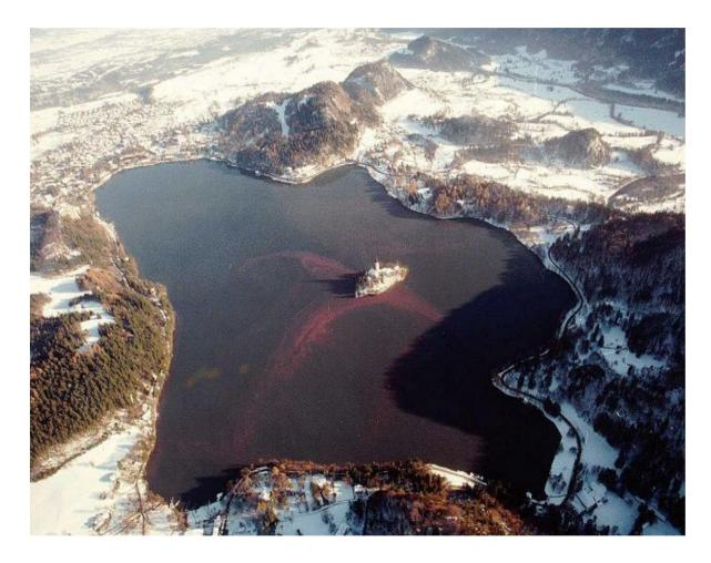
Vol. =  $25.7 \times 10^{6} \text{ m}^{3}$ Area =  $1.47 \times 10^{6} \text{ m}^{2}$ Max. depth = 30 m(western basin) Avg. depth = 17.5 m
