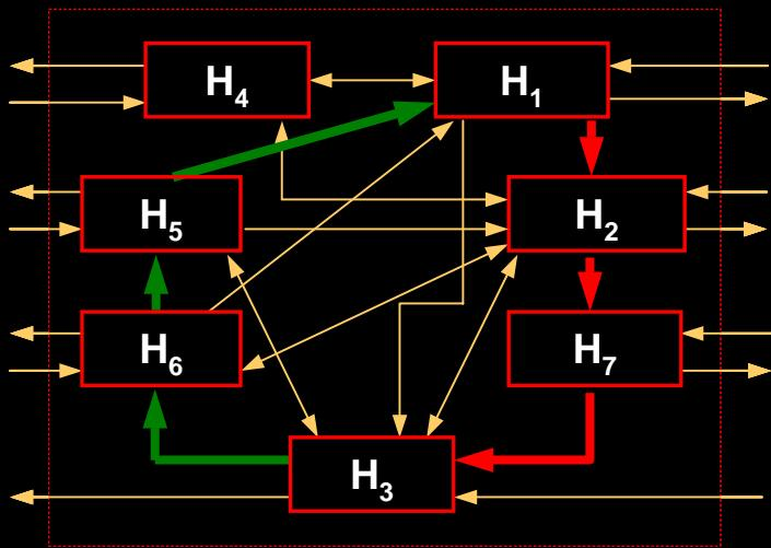
Example: Quantity of paths of length,  $m = 3$ , between  $H_1$  and  $H_3$
